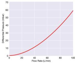
\*The flow/pressure drop characteristics refer to the empty housing only for water at 20°C. For other liquids multiply pressure drop by relative density. To obtain the total pressure drop of a complete filter assembly, the cartridge pressure drop must be added.
